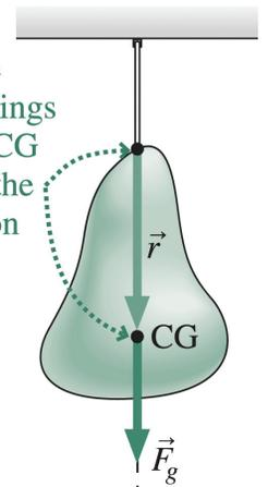
Measuring the center of gravity
