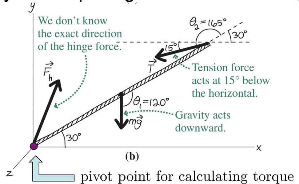
Torque due to tension  $\vec{T}$ :  $\tau_T = LT \sin(165^\circ)$
