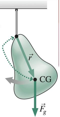
. . . so the object swings until the CG is below the suspension point.
