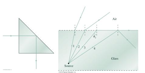
TIR is the basis of optical fibers, guiding light along the fibers that, among other applications, carry data on the interwebz.
