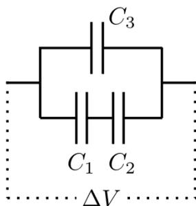
2. Consider the above arrangement of capacitors, where  $C_1 = 2.0 \mu\text{F}$  and  $C_2 = 2.0 \mu\text{F}$  are in series, and  $C_3 = 1.0 \mu\text{F}$  is parallel to the series combination.
