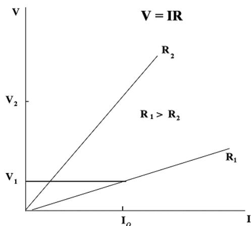
If the voltage across an “Ohmic” resistor is increased, a graph of voltage  $V$  versus current  $I$  shows a straight line (indicating a constant resistance). **The slope of the line is the value of the resistance.** However, if the resistance *changes* (that is, if the resistor is “non-Ohmic”), the graph of voltage versus current will not be a straight line. Instead, it will show a curve with a changing slope.
