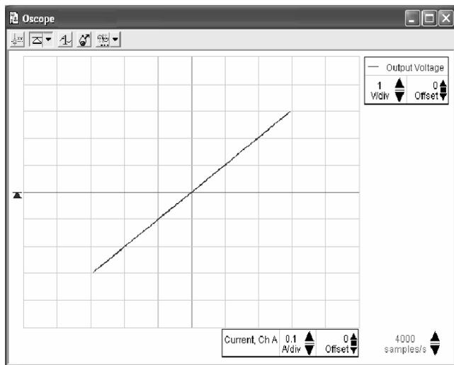
• The figure on the left shows a typical output of the experiment. The vertical axis is the voltage  $V$ , while the horizontal one is the current  $I$ .
