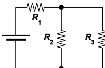
2. (5 pts). In this experiment for the resistors in parallel circuit configuration, if we added to the circuit two additional parallel legs with each leg having a single  $50\ \Omega$  resistor, what would be the new **theoretical total resistance** of the circuit? Show your work.
