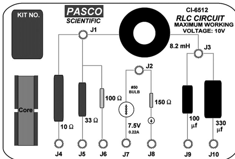
**NOTE: The RLC jack points are not directly numbered on the board; refer to the figure on the left.**
