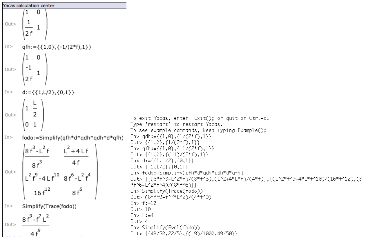
Figure 3: A simple FODO cell calculation in the web interface (left) and terminal interface (right) to yacas. The terminal interface example also shows numerical evaluation.
