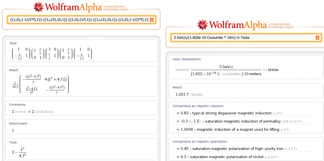
Figure 2: A simple FODO cell calculation, and a calculation of required magnetic field to bend a q = e , p = 3 \text{ GeV}/c particle through a bending radius of \rho = 10 \text{ m} in Wolfram Alpha.
