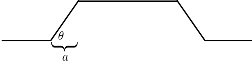
Figure 1: A simple four-dipole chicane, with no quadrupoles.
