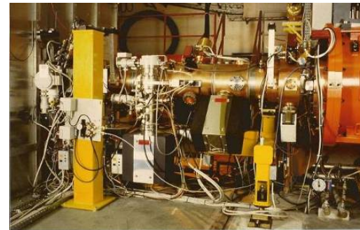
The new RFQ2 pre- injector at CERN (1993): Source+LEBT +RFQ
