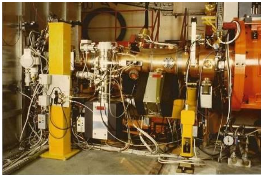
Fig. 3: The new 750 keV RFQ2 (1993) installed in front of CERN Linac2
