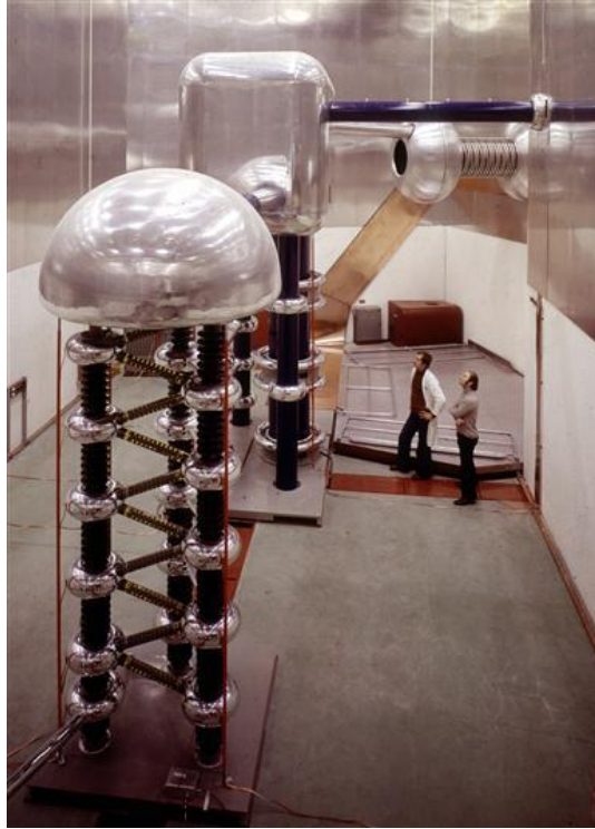
Fig. 1: The old (1976–1993) HV installation of CERN Linac2, with the 750 kV Cockcroft–Walton in the front, the ion source electronics in its HV cabin in the background, and the sphere containing the proton source and the HV insulation to the right. The linac is in another room to the right.
