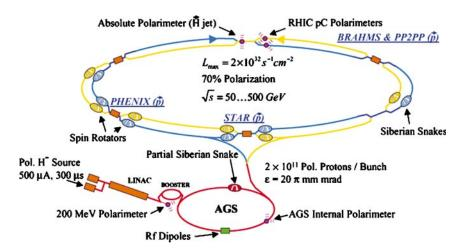
Figure 22 Layout of the Brookhaven accelerator complex with expected performance goals.
