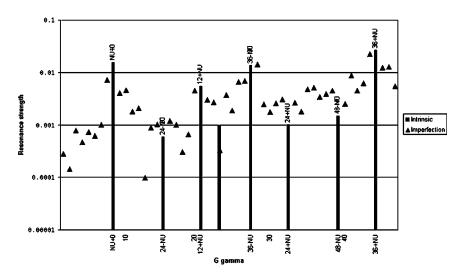
Figure 20 Depolarizing resonances, intrinsic and imperfection, in the AGS.
