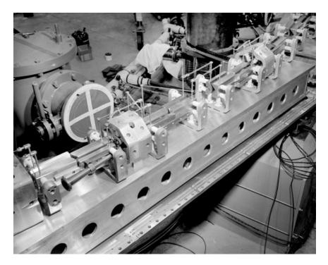
**Figure 12** Section of the electron analog showing electrostatic dipole and quadrupole lenses.
