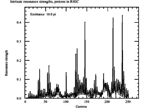
Figure 21 Intrinsic depolarizing resonances in RHIC.
