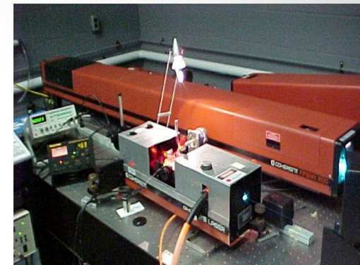
Argon ion laser (257.3 nm) frequency doubled
