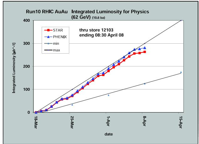
Figure 5: Integrated luminosity for RHIC operation at 31.2 GeV.
