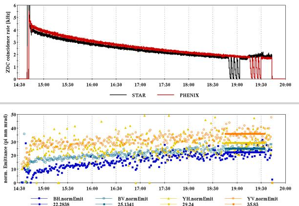
Figure 2: Store 12081 during the 31.2 GeV run with two vernier scans at the end. ZDC coincidence rate (top) and IPM emittance measurements (bottom).
