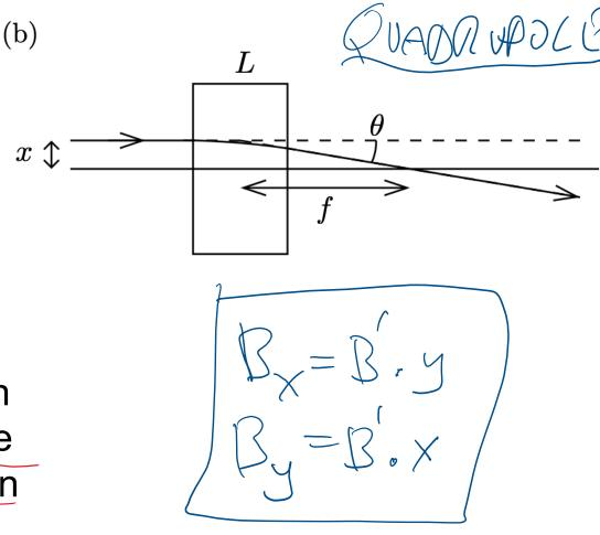
2.6 Motion through an iron quadrupole, focusing in the horizontal but defocusing in the the vertical.
