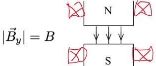
2.5 Motion through a dipole with a constant vertical field B.
