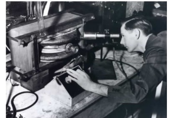
Donald Kerst UIUC 2.5 MeV First Betatron, 1940 NOT sync radiation!
